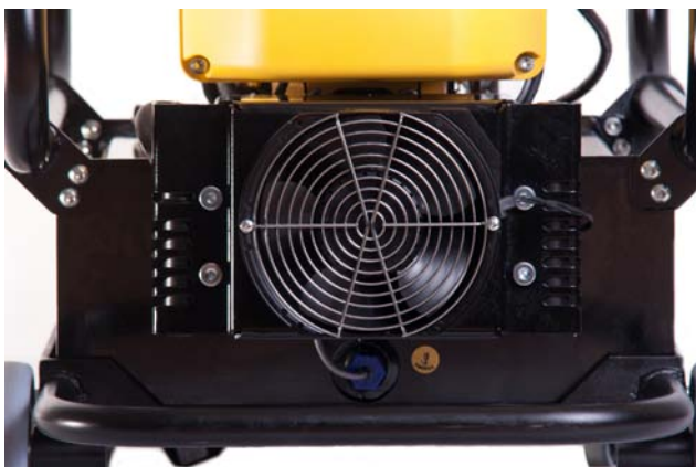
Reservoir heat exchanger
